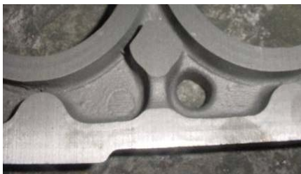
No veining in the water-jacket area.
