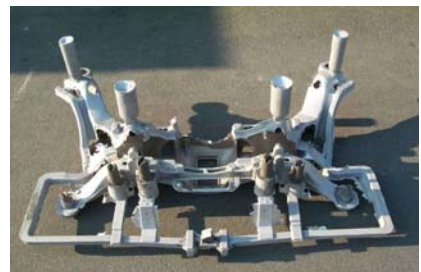
Smoother filling pattern with lower metal velocities created
