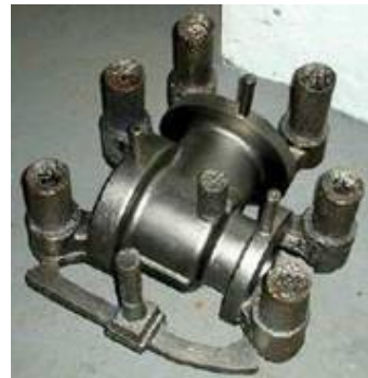
Redesigned gating system with STELEX ZR ceramic foam filter at base of downsprue in filter position FP 7
